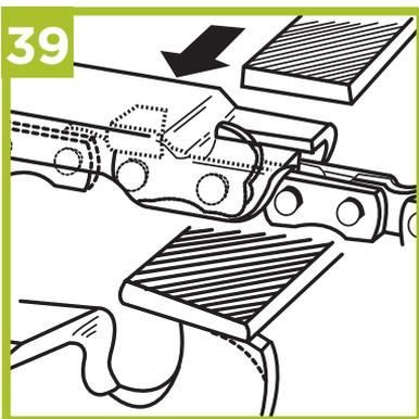
After sharpening, the cutting links must all have the same width and length.
